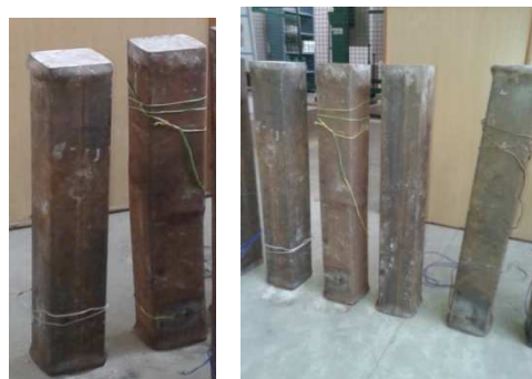
Figure 15: Failure Mode in Silica Fume Infilled Column
