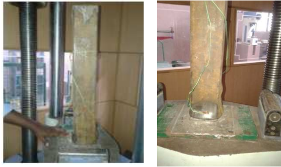
Figure 13: Failure Mode in M30 Infilled Column
