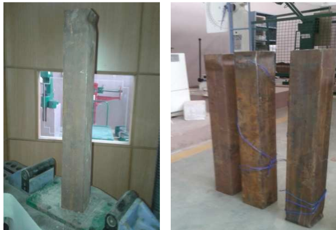
Figure 11: Failure Mode in Hollow Column
